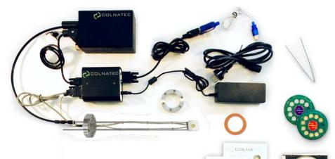
Contributing to the accuracy of this temperature control system are a built-in thermocouple that conveys temperature data to the Eon™ controller - which makes realtime adjustments to the heater - and the Mirage™ air-cooling unit, which automatically delivers supercooled compressed air into the sensor in response to the fluctuating temperature changes of the sensor.
