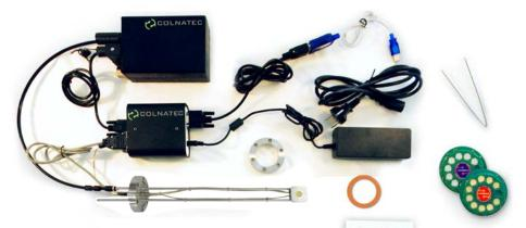
Contributing to the accuracy of this temperature control system are a built-in thermocouple that conveys temperature data to the Eon<sup>™</sup> controller - which makes realtime adjustments to the heater - and the Mirage<sup>™</sup> air-cooling unit, which automatically delivers supercooled compressed air into the sensor in response to the fluctuating temperature changes of the sensor.
