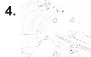
**4.** Press sensor head and feedthrough flanges together. Align bolt holes. Apply bolts and plate-nuts. Tightening bolts compresses copper gasket between a sharp edge and a tapered groove, creating a near-perfect seal.
