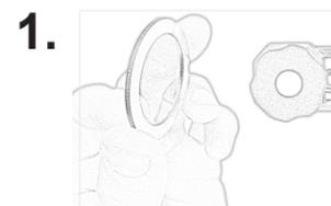
**1.** Obtain a copper Conflat™ gasket and place onto sensor head.
