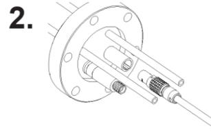
**2. Connect Heater Control Cable to Tempe™**
