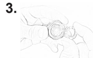
**3.** Remove retainer ring to access mock crystal using supplied tool.
