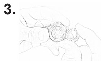
**3.** Remove retainer ring to access mock crystal.
