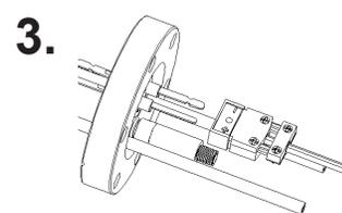
**3. Plug Phoenix™ TC Connector into Socket of TC Extension Cable (If using TC-equipped Monitor)**
