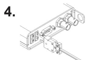
**4. Plug TC Adapter into TC Female Socket of Monitor (If using TC-equipped Monitor)**
