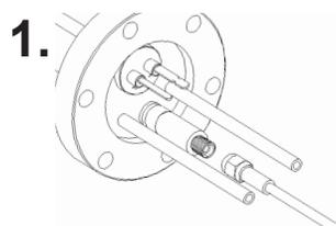
**1. Connect SMA Coaxial Cable to Phoenix™**
