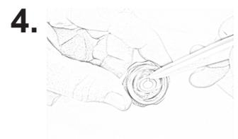
**4.** Remove mock crystal from sensor head cap (use a non-metallic tool).
