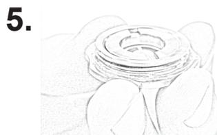
**5.** Place the threaded side of the retainer ring onto the corresponding threads of the sensor cap. Tighten the retainer ring by turning the ring COUNTER CLOCKWISE.
