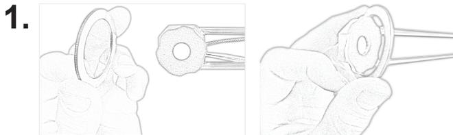
1. Remove copper gasket from packaging and thread onto sensor head.
