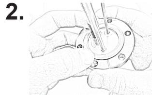
2. Fit gasket into circular groove on Conflat.
