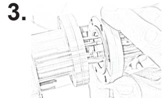
3. Hold copper gasket in place while inserting sensor head into chamber feedthrough.
