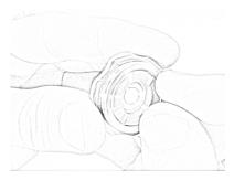
4. Remove mock crystal from sensor head cap.
