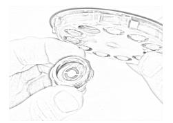
4. Use a plastic prod to adjust crystal position until crystal rests snugly in the crystal seat.
