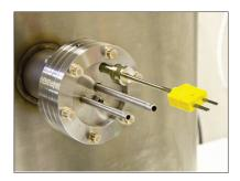
**WARNING** Hand-tighten flange bolts before using wrench, alternating among bolts and using a sequential torque pattern.
