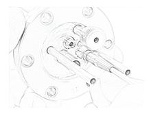
Connect Phoenix<sup>™</sup> to Eon-LT<sup>™</sup> Connect BNC extension cable to SMA, which then connects to the BNC adapter cable using the provided BNC union. Then, connect the other end of the BNC extension cable to the Eon-LT<sup>™</sup> coaxial input (either sensor 1 or 2).
