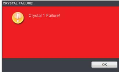
Although it is recommended that the sensor alerts generally remain enabled, the user can disable the notifications in the instance that the crystal is being used in a testing environment.
